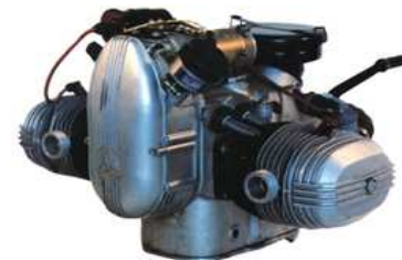
OHV(12V 32HP, over head valve) Engine
